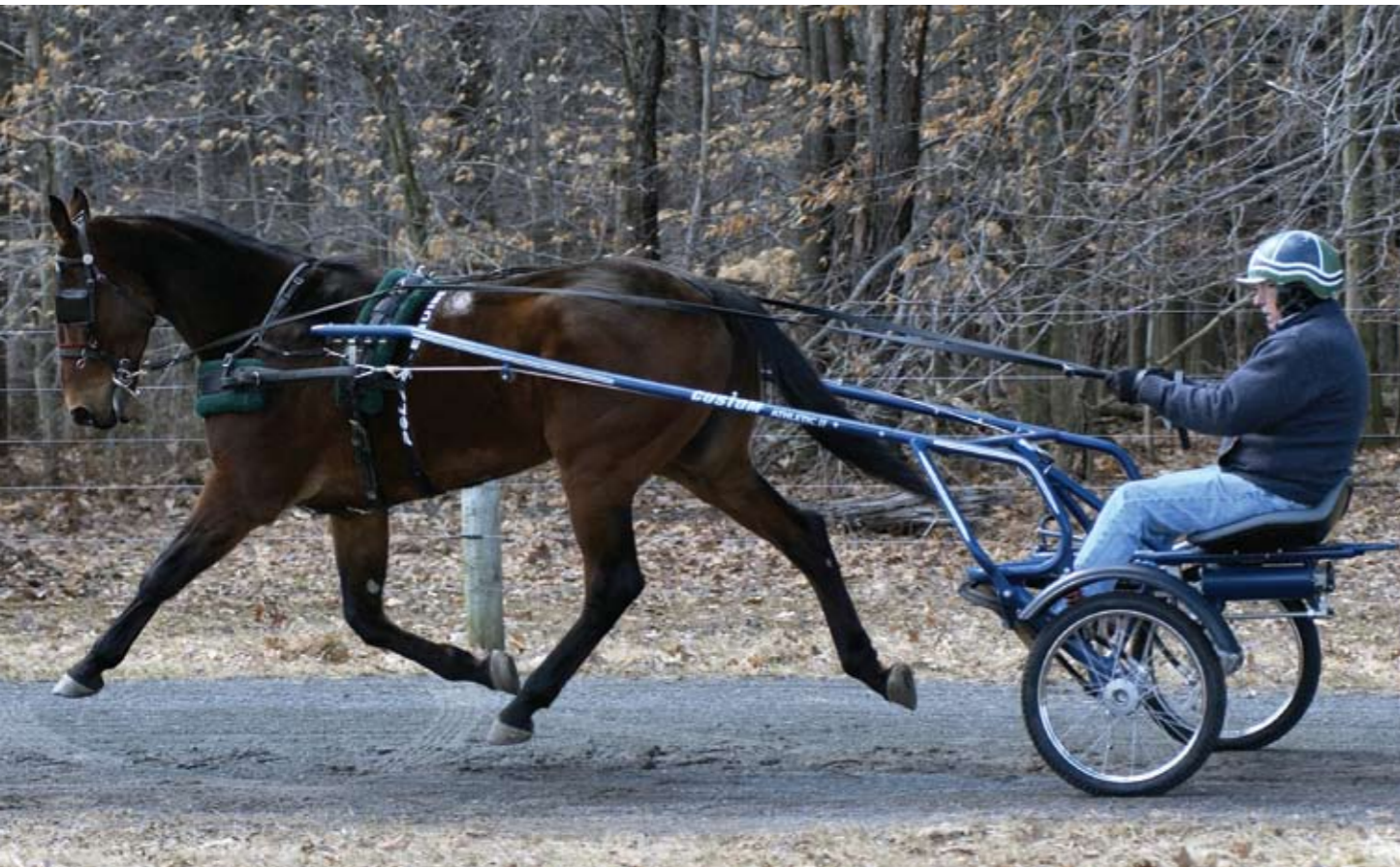
The cart is very well balanced, so the horse doesn't feel the weight of the cart. The resistance is against the wheels not against a horse's joints.
